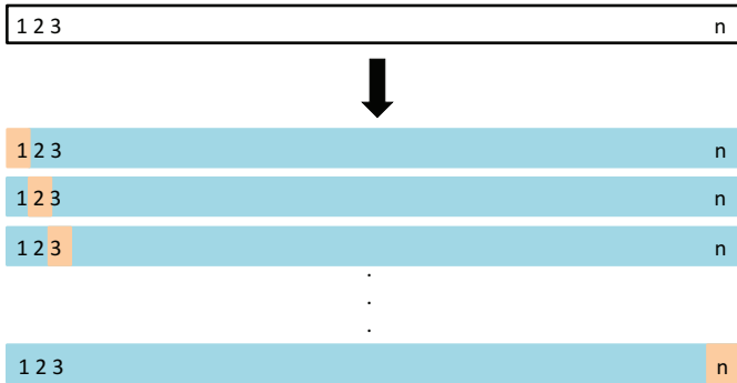
FIGURE 5.3. A schematic display of LOOCV. A set of n data points is repeatedly split into a training set (shown in blue) containing all but one observation, and a validation set that contains only that observation (shown in beige). The test error is then estimated by averaging the n resulting MSE's. The first training set contains all but observation 1, the second training set contains all but observation 2, and so forth.
